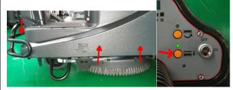
To uninstall the brush, the deck must be in high position and just push on the button.
