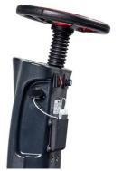
USB plug to charge mobile during working time of the machine.
