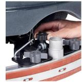
Turn the screw on the arm of the squeegee to adjust picking water on the rear squeegee.
