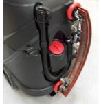
For storing the squeegee you can attached it on the back of the machine.
