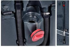
On the back of the machine, full fill in water up to 72 liters and add detergent.
