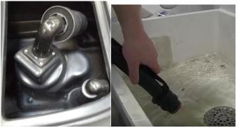
Emptying the tank of dirty water and rinse it. Remove the floating system and rinse the ball inside. Keep it clean.
