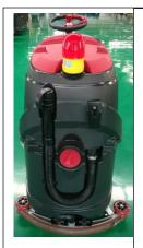
Turn on the flashing light during the cleaning of the floor and during the transport of the machine.
