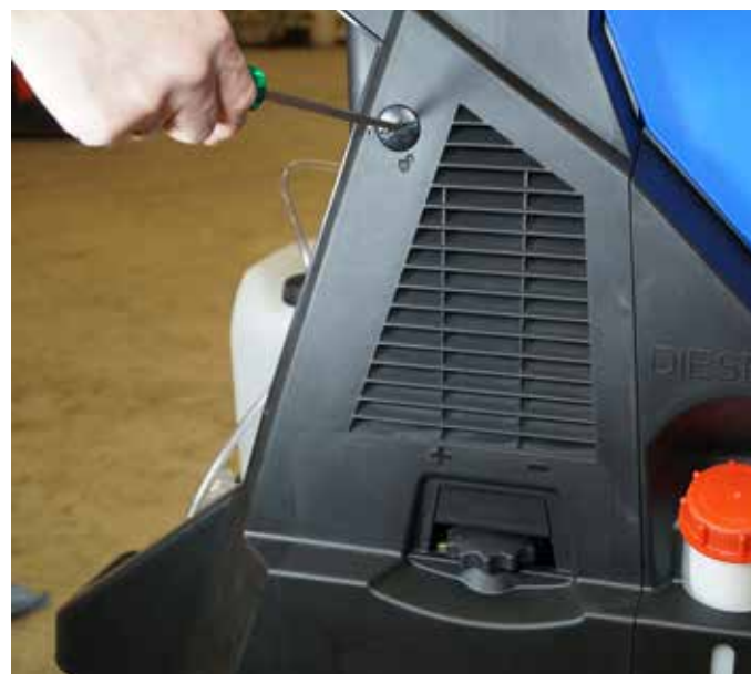
1. Open service door by turning quarter turns.
